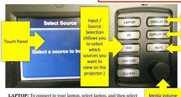
**LAPTOP:** To connect to your laptop, select laptop, and then select Analog or Digital Input based on the type of connector you are using. (See picture to the right.)
