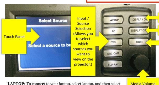
**LAPTOP:** To connect to your laptop, select laptop, and then select Analog or Digital Input based on the type of connector you are using. (See picture to the right.)
